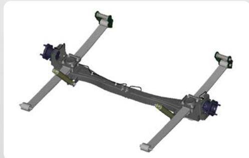
Rigid & Semi-elliptic Leaf Spring rear suspension.
