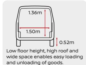
Low floor height, high roof and wide space enables easy loading and unloading of goods.
