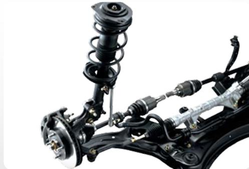
Independent MacPherson strut front suspension with stabiliser bar.
